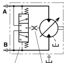
Hydraulic schematic - V14 with built-in flushing valve.
