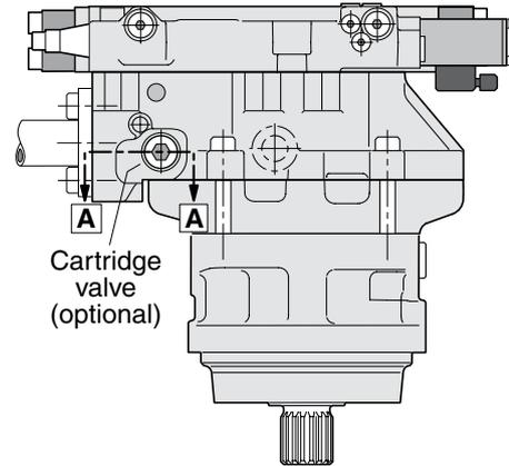
V14- 110 (EP control) with relief valve cartridges.
